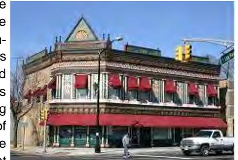
floor façade is made up of rectangular raised panels that hold the plate glass display windows. Windows on the first and second floors of the pressed metal section are separated by decorative pilasters with floral designs. The south side elevation is made of simple tan brick with the same decorative cornice.
